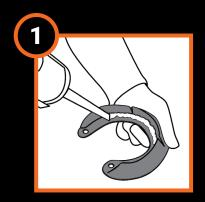
Put a medium bead of Shufit glue around the inside base of the shoe and cuff.
