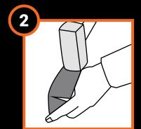
To reshape GluShu, hit the desired area with a hammer.
